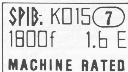
Figure 6. Samples of Machine Stress Rating (MSR) stamps used on lumber.
