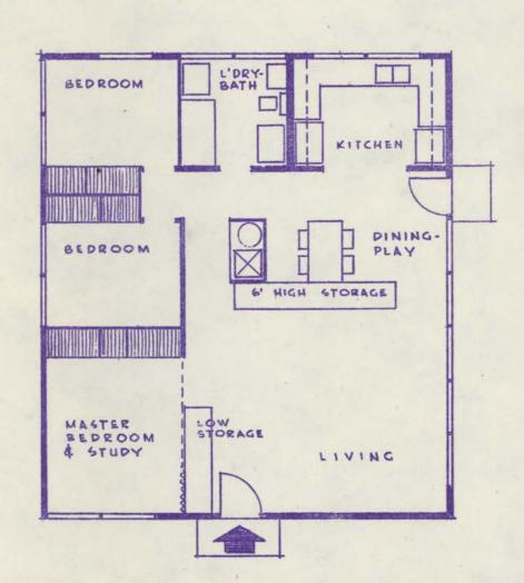
Variation #7 is a three-bedroom utility-core plan. All plumbing and heating equipment, with the exception of the kitchen sink, is included in a single central block. The bedrooms are arranged along one side of the plan, and the living and dining areas are on the opposite side, separated from each other by a 1-foot deep storage unit. The dining area is large enough to be used also as a play area, with easy access to outdoor space which can be supervised from the kitchen.
