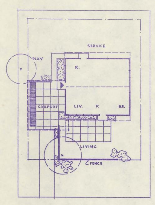
Variation N-2 is oriented in the same way as N-1, but in this scheme the garage or carport is placed towards the rear of the house, and the house is moved up to the building setback line. For the sake of privacy, the sill line of the south-facing windows is raised to 31-4" above the floor.
