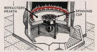
THE POT-TYPE BURNER IS QUIET IN OPERA-TION, BUT REQUIRES CLOSE ADJUSTMENT
