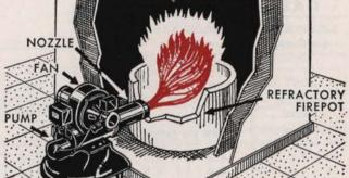
ROTARY BURNERS CAN BE USED SUCCESS-FULLY WITH LOW OIL FEED RATES
