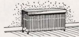
CAST-IRON RADIATOR WITH SHIELD
