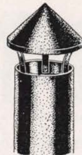
METAL OR ASBESTOS CONE-TYPE TOP
