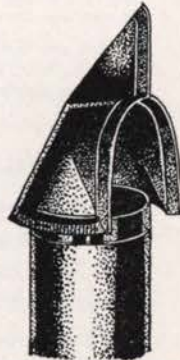
ROTATING METAL CHIMNEY TOP
