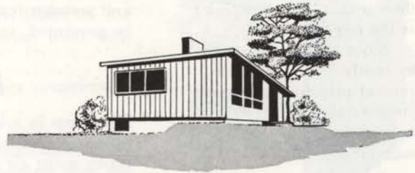
A level lot can be graded so that the front of the house has a low-to-the-ground appearance, while basement windows at the sides and rear are above grade level.
