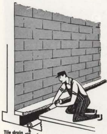
A tile drain installed under basement floor relieves water pressure.
