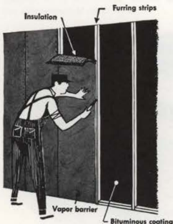
Insulation helps to keep basement walls warm; thus, water vapor does not condense on them readily.
