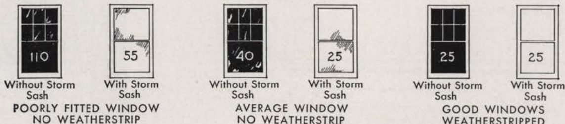
Figures on Windows Indicate Cubic Feet of Air Leakage per Hour for Every Foot Length of Crack Around Sash
