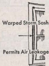
RESULT OF WARPAGE IN STORM SASH
