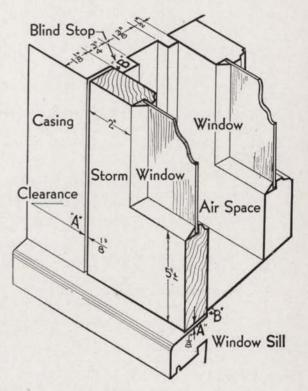
e. Proper Clearance for Fitting.—Storm windows should have a definite clearance between sash and window frame of about 1/8". If no clearance is provided, any swelling of the sash will bind it in the frame and may cause it to warp and become leaky.
