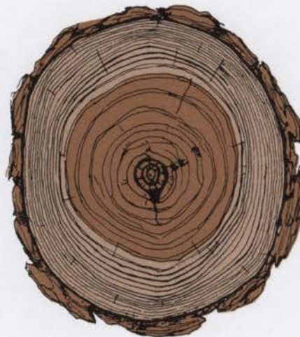
Tree Cross-section: Heartwood is generally more resistant to decay than sapwood; sapwood accepts chemical treatment more readily.
