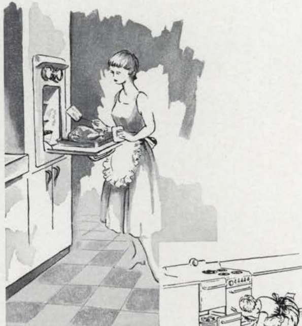
The separate oven can be placed at a convenient working height.
