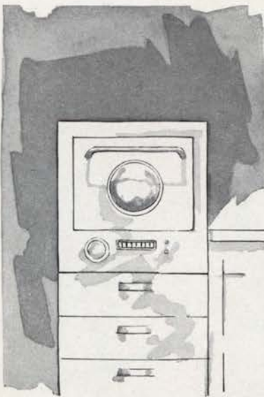
If the oven has a finished exterior, it can be incorporated directly into the kitchen assembly. Storage cabinets or drawers can be placed below the oven.
