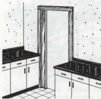
Sliding doors do not block cabinets.
