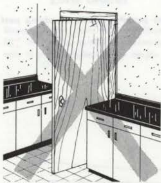
Doors swinging into kitchen are not desirable.
