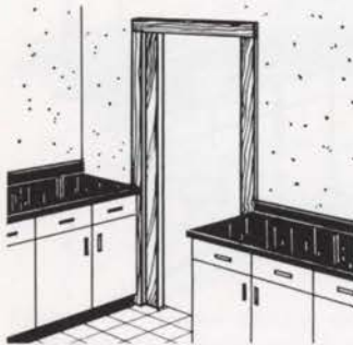
Sliding doors do not block cabinets.
