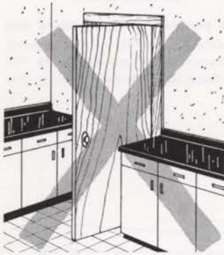
Doors swinging into kitchen are not desirable.
