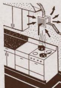
FAN INSTALLATION WHEN RANGE IS NEXT TO OUTSIDE WALL
