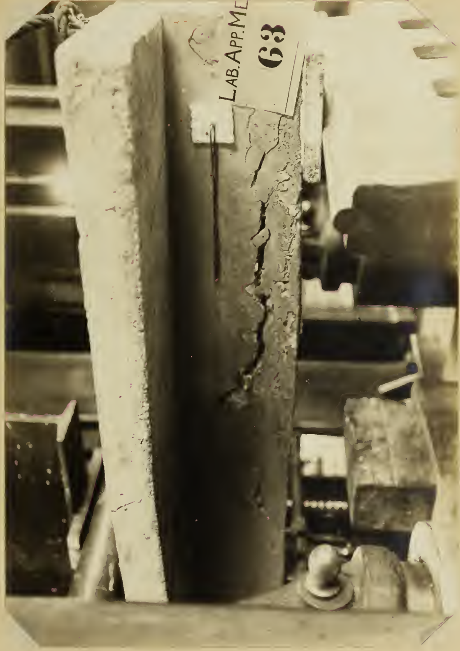
T-Beam No. 23 Showing Failure by Diagonal Tension.
