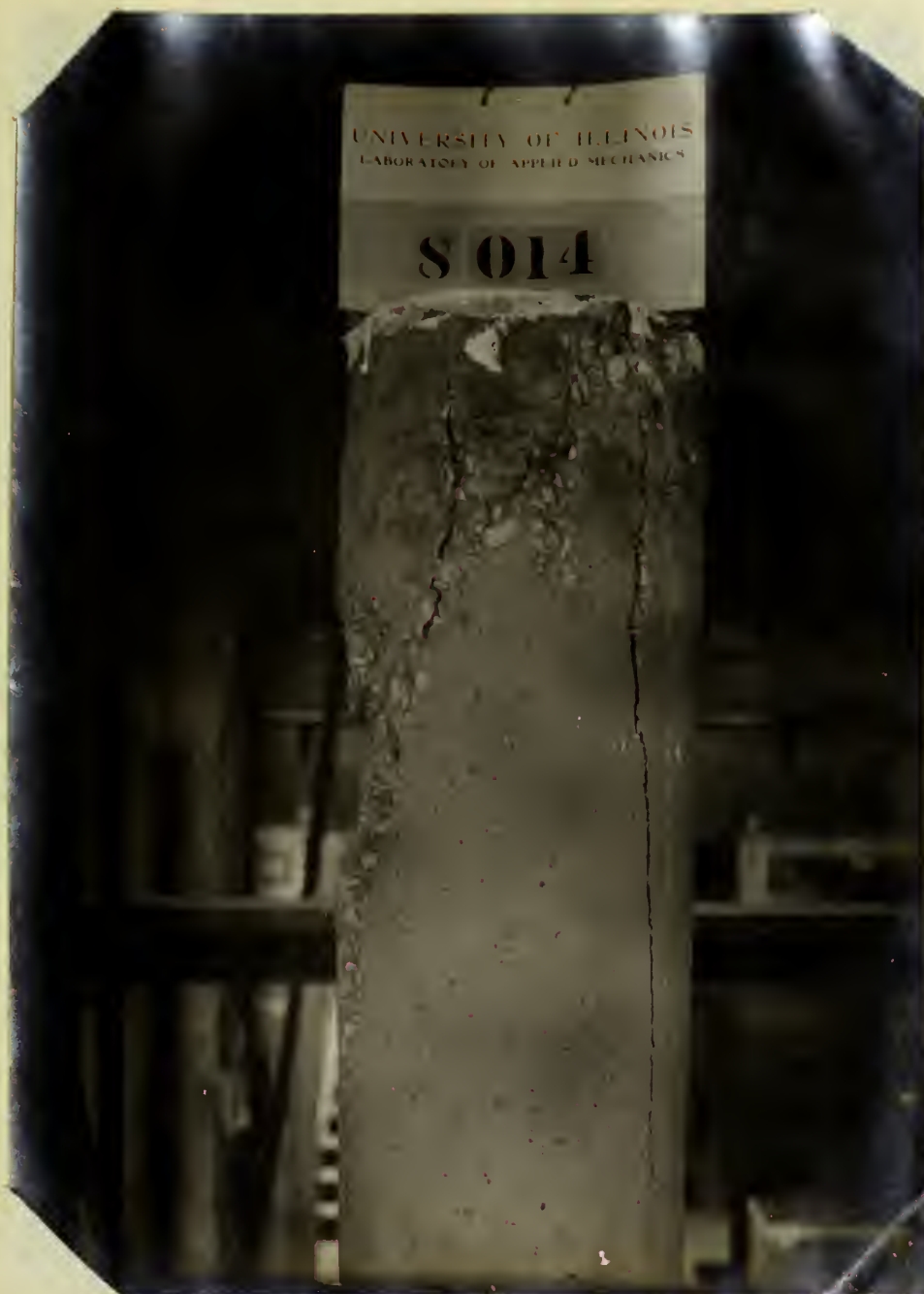
View Showing Crushing in Connection with Shearing Failure.
