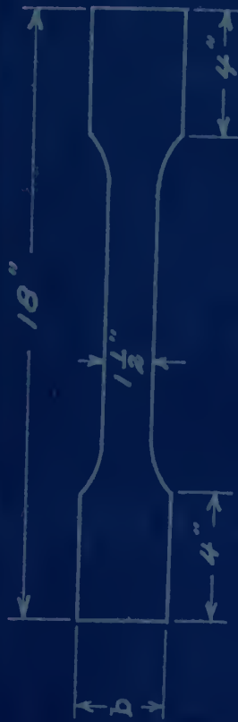
b, width of test piece
