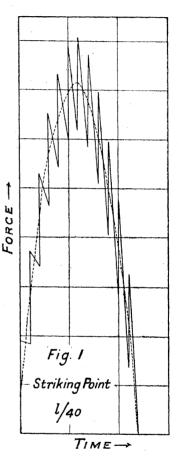
contact in a continuous manner, so long as the number of discontinuities in the graph remains unaltered. At the successive stages, however, at which the number of discontinuities in the graph decreases by unity, the duration of contact *decreases* by a finite amount in a discontinuous manner, these jumps being the greater and further apart, the more distant the striking point is from the end.
