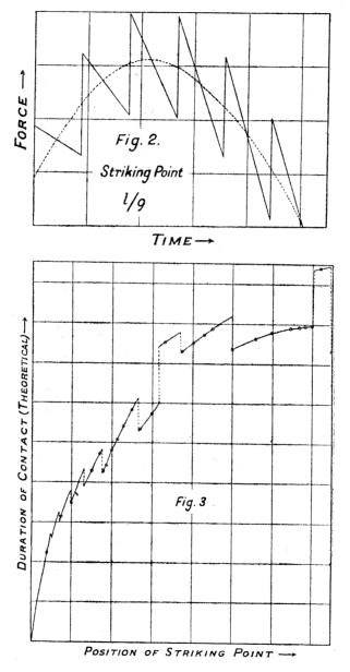
point, and the latter when it goes down by the same amount. The whole course of values for the duration of contact for 27 different positions of the striking point between the end and centre of the string is shown in fig. 3.
