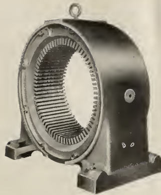
Primary Ready for Winding.
