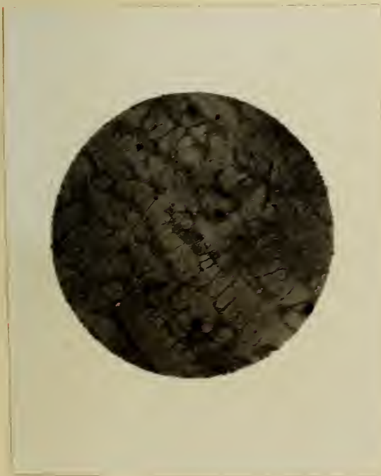
Fig. 9 Cu-Cr w. 0.31% Cr. Cooled slowly. Unetched. Hypo-eutectic w. excess Cu. x80.
