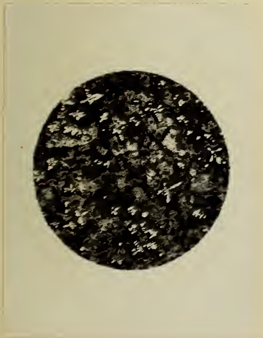
Fig. 21. Cu-Cr w. 4.69% Cr. Quenched from molten state by pouring directly into water. x80.
