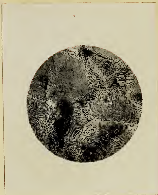
Fig. 12 Cu-Cr w. 0.43% Cr. Cooled Slowly. Etched w. HNO_3 . Structure near eu- tectic. Large crystalline grains on outer edge. x210.
