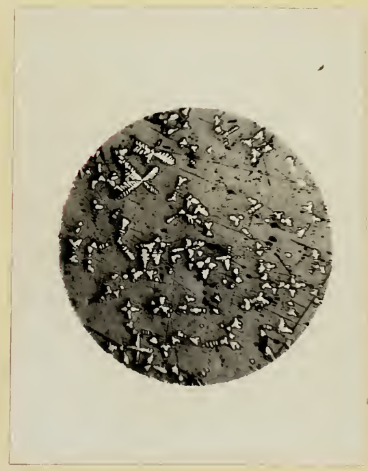
Fig. 22 Cu-Cr w. 4.83% Cr. Cooled slowly. Unetched. Well formed dendrites of Cr. x80.
