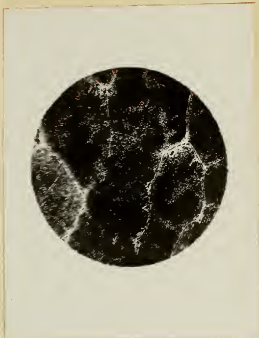
Fig. 16 Cu-Cr w. 0.46% Cr. Quenched. Etched w. dil. \text{HNO}_3 . Showing boundaries of crystalline grains. x80.
