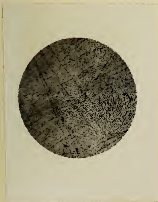
Fig. 13 Cu-Cr w. 0.43% Cr. Same as in Fig. 12. x210.
