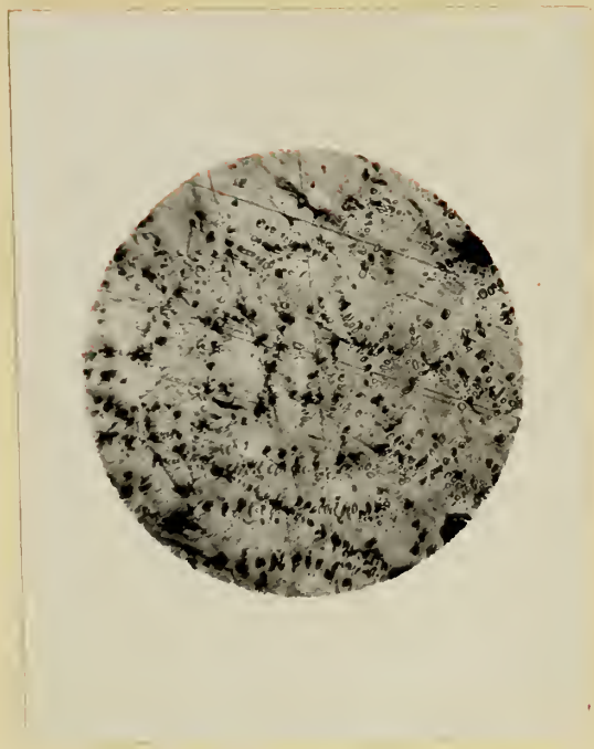
Fig. 20. Cu-Cr w. 2.61% Cr. Cooled slowly. Hyper-eutectic structure. Porous. Excess chromium showing. x80.
