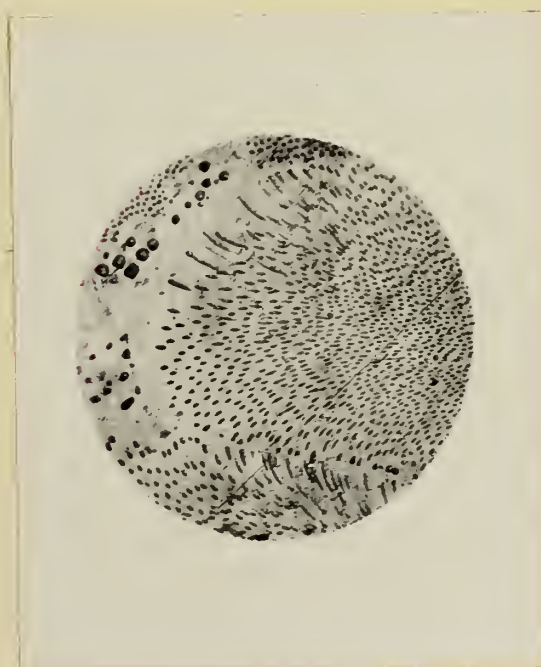
Fig. 14 Cu-Cr w. 0.43% Cr. From same specimen as Fig. 12. x210.
