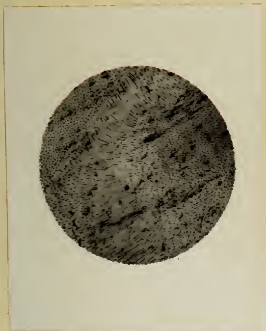
Fig. 15 Cu-Cr w. 0.43% Cr. Showing rod-like structure in eutectic. x210.
