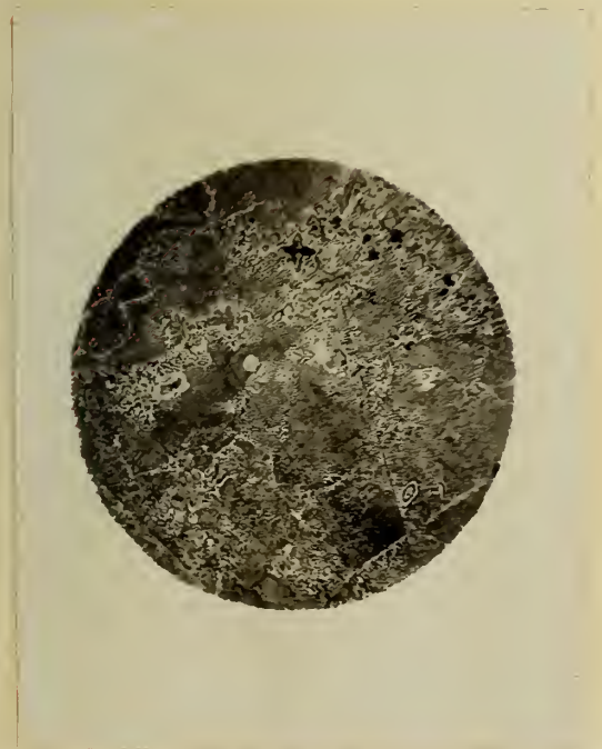
Fig. 17 Cu-Cr w. 0.46% Cr. Same as Fig. 16. Quenched. Etched w. \text{I}_2 in \text{C}_2\text{H}_5\text{OH} . x80
