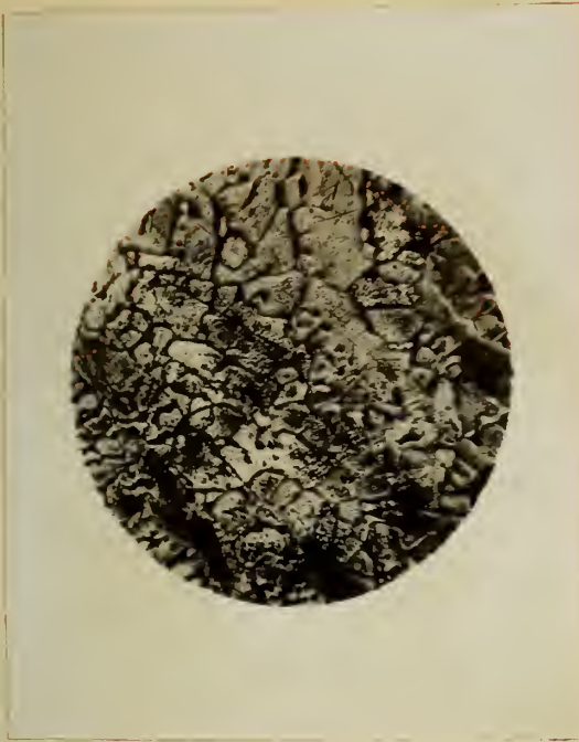
Fig. 7 Cu-Cr w. 0.16% Cr. Cooled slowly. Etched w. dil. \text{HNO}_3 . Polyhedral crystals from center of specimen. x80.
