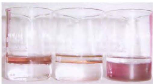
Figure 6. (Middle) Nanocrystals of Au formed at the toluene–water interface. (Left) When dodecanethiol is added to the toluene layer, the Au nanocrystals form an organosol. (Right) When mercaptoundecanoic acid is added to the water layer, the Au nanocrystals produce a hydrosol.
