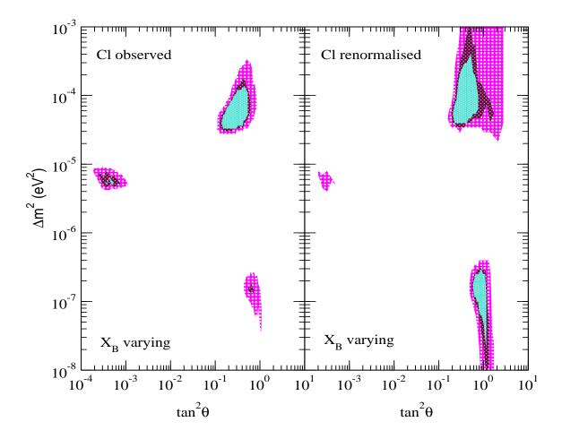
**Fig. 3**: The 90, 95 and 99% C.L. allowed area from the global analysis of the total rates from Cl (observed and 20% renormalised), Ga and SK detectors and the 1117 days SK recoil electron spectrum at day and night, assuming MSW conversions to active neutrinos. The B normalisation is floated as a free parameter.
