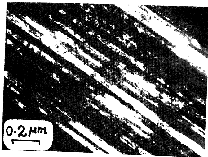
Figure 4. Dislocation sub-bands in severely cold-worked niobium-titanium alloys.
