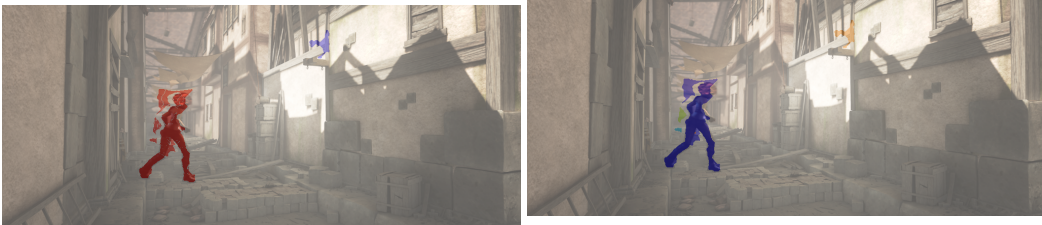
Predicted Current Segmentation by adding the optical flow of previous frame to previous image frame seg_{i-1} + flow_{i-1} Predicted Segmentation with Cracks Filled
