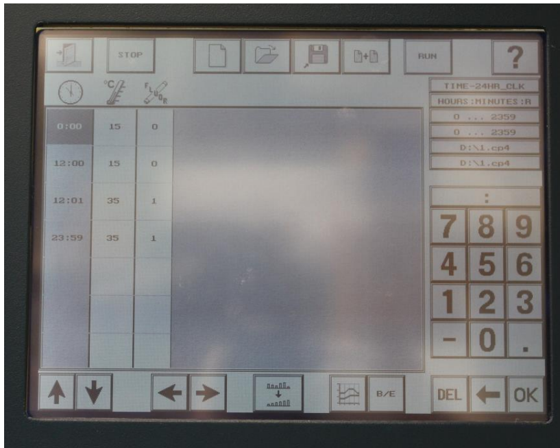
Figure A.3: Germination chamber screen showing correct settings for germinating waterhemp.
