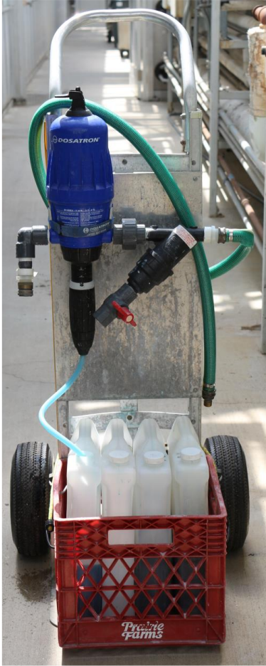
Figure A.7: The Dosatron cart used for liquid fertilizer application. Users should ask for help from a member of the Plant Care Facility staff prior to operating for the first time. The 20-20-20 concentrate option is what is normally used for waterhemp.
