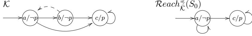
Figure 5.6: An LKS \bar{\mathcal{K}} with S = \{a, b, c\} , S_0 = \{a\} , and \mathcal{L}(c) = \{p\} , and its folded abstraction \text{Reach}_{\bar{\mathcal{K}}}^{\preceq}(S_0) , where the dashed arrow denotes b \preceq a .
