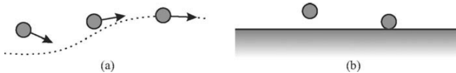
Figure 2.1: (a) Guidance virtual fixture. (b) Forbidden-region virtual fixture [5].
