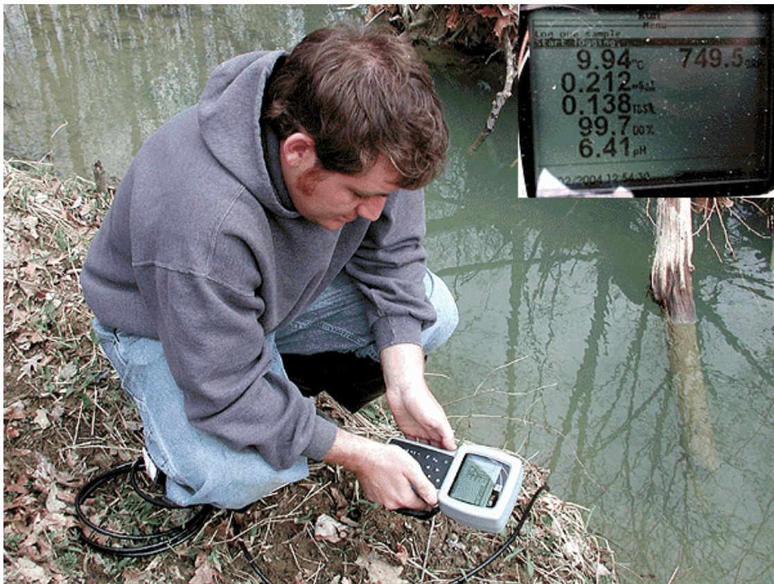
Figure 5. A) Using flow meter to determine volume of flow, B) placing water sample in turbidity meter, C) using YSI multimeter to collect various water quality parameters – inset shows detail of display.
