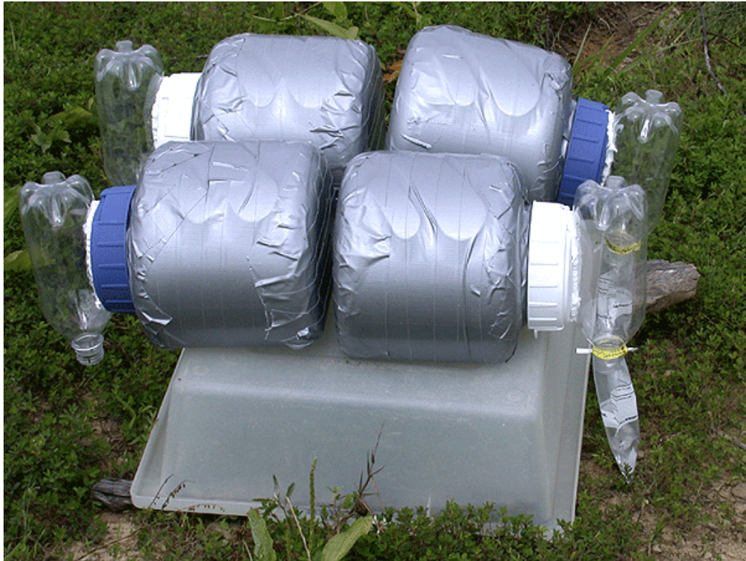
Figure 7. Four “photo tactic optimal insect extractors” (PTOIEs) in operation. Sweep sample material is placed in darkened (duct-tape covered) chambers. Diurnal, positively phototactic insects are attracted to light coming from hole in lid, and eventually fall into the whirl pack bag, below, where they are preserved.
