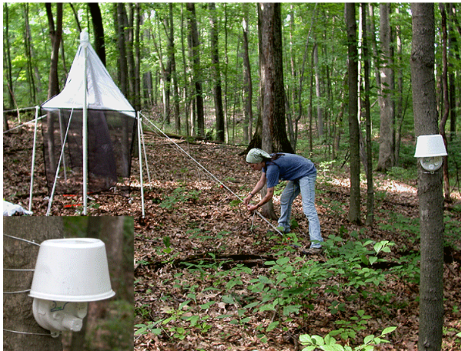
Figure 18. HOBOPro RH/Temp Data Logger mounted on tree (foreground and inset) at forested site F5 on 6 July 2004. Malaise trap is being set up in background.
