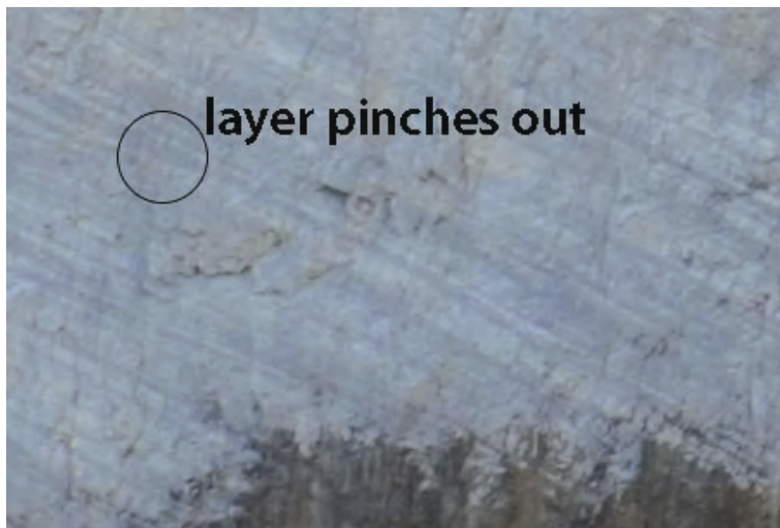
Figure 14 Change in bedding thickness and continuity at the north flank site. Circle shows where a light-toned bed exhibits pronounced change in thickness. The light-toned bed pinches out completely. Note the dark algae and stains from groundwater on the lower edge.
