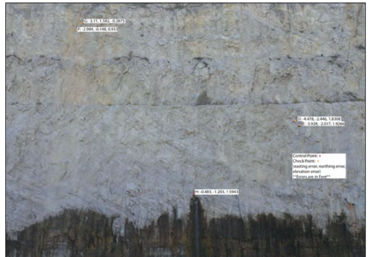
Figure A4.9 Control point H immediately above a small cave issuing water and check points for orthophotograph 3008-3009. Errors are shown in feet for easting, northing, and elevation.
