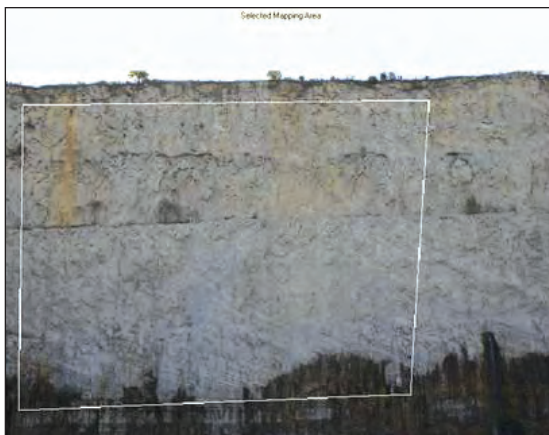
Figure A1.10 Four points are selected on one of the stereopair photographs to delineate the 3-D model output extent.
