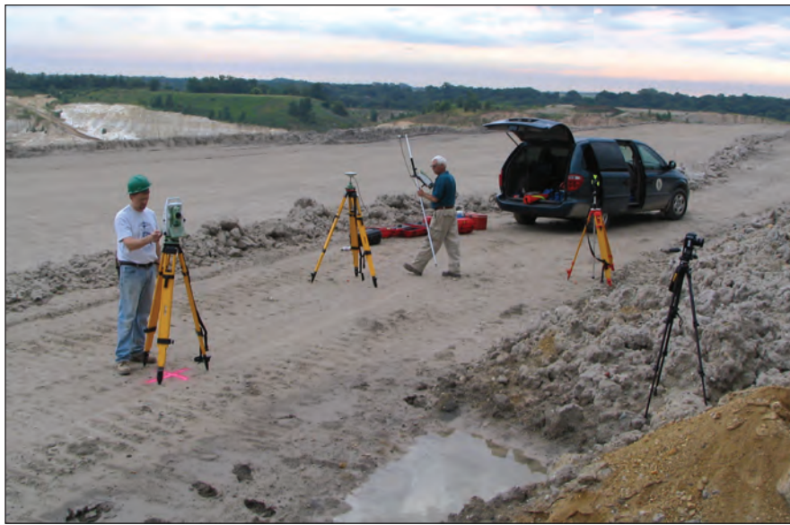
Figure A1.3 Typical field setup with a total station and operator (left), GPS base station (middle), and RTK GPS rover (carried by operator), backsight prism (right), and camera (foreground). Photographs for stereomodels are spaced 1/7 of the distance between the outcrop and the camera station.
