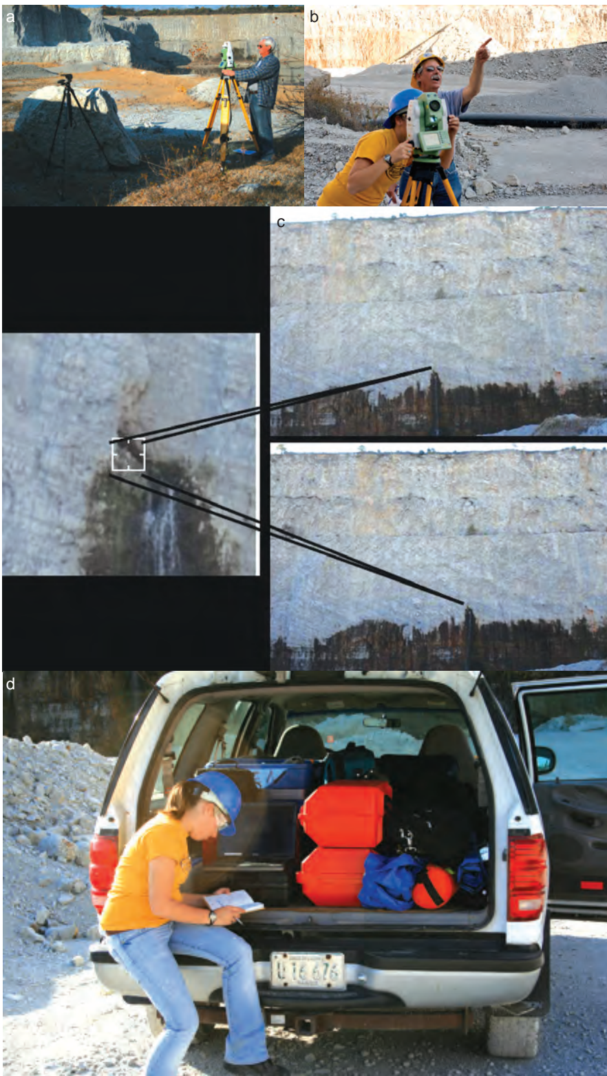
Figure 5 Surveying the camera station (a) and the reference mark on quarry wall (b and c) and noting the mark location on the photomosaic on a notebook computer (d).
