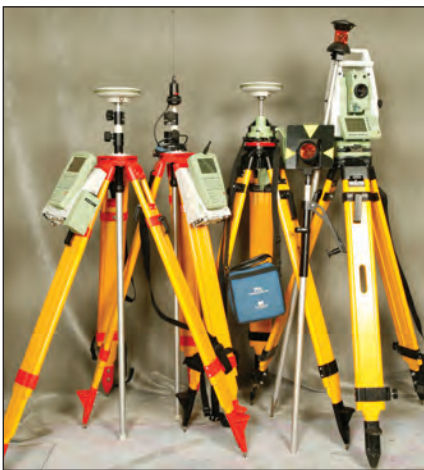
Figure A1.1 Leica 1200 Total Station (right) and RTK GPS (center and left).
