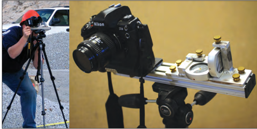
Figure A1.2 Recording a tilted image using a specially built bracket devised by Michael Dodd at the ISGS. The Nikon D80 camera is mounted on the tripod and Dodd bracket with compass and clinometer (right). The clinometer is on the left of the bracket, the compass is in the middle of the bracket, and the camera mounting plate is to the right.
