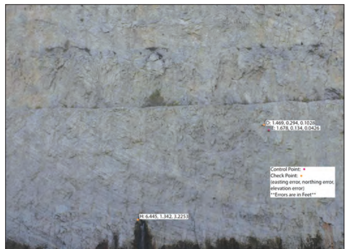
Figure A3.9 Control point E and check points for orthophoto-graph 3007-3008. Errors are shown in feet for easting, north- ing, and elevation.
