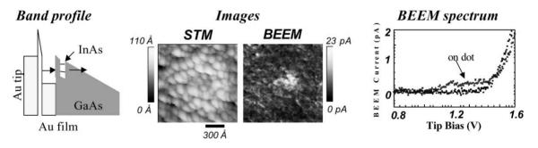
Fig. 48. (from left to right) Schematic of band profile, STM and BEEM images, and characteristic BEEM spectra for InAs/GaAs self-assembled single quantum dots [38].
