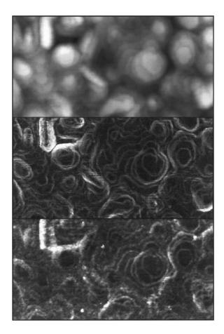
Fig. 29. STM and BEEM images of a 200 Å Au/Si(100) sample. The 100 nm × 350 nm images are obtained at  $V_t = 1.1$  V and  $I_t = 1$  nA. The top image is the STM surface height (17 Å white to black), the middle image is its calculated surface slope, and the bottom image is a map of BEEM current,  $I_c$ . The mean BEEM current is 2.25 pA, and total range shown is 2.4 pA. BEEM contrast is about 30% [93].
