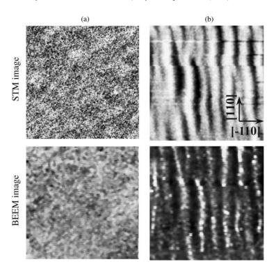
Fig. 36. Room-temperature 1  $\mu$ m × 1  $\mu$ m STM image (top) and BEEM image (bottom) of GaAs/GaInP<sub>2</sub> layer grown by MOCVD on (a) (511) n-GaAs substrate, (b) on n-GaAs substrate misoriented by 6° to [111]<sub>B</sub>. A tip bias is -1.7 V and a tunnel current is 4 nA [16].
