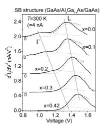
Fig. 14. Room-temperature SD-BEEM spectra for five different Al compositions (solid lines). For clarity, the SD-BEEM spectra are shifted along the vertical axis. Thin solid lines are eye-guides for the peaks position development. The MSIS model calculations are also presented. The model calculations show the separate  $\Gamma$  and L valley contributions (dotted lines) and their sum (dashed lines) [5].
