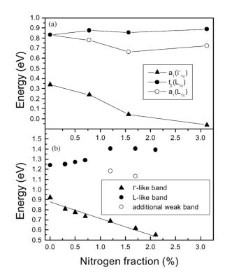
Fig. 39. (a) First-principles LDA calculations of the  $\Gamma_{1c}$  and  $L_{1c}$  compositional dependencies of GaAs<sub>1-x</sub>N<sub>x</sub>. (b) The compositional dependencies of the thresholds observed in the SD-BEEM spectra of GaAs<sub>1-x</sub>N<sub>x</sub>. The solid line is the best linear fit to the  $\Gamma$ -like threshold giving a slope of -16.4 eV [20,164].
