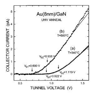
Fig. 35. BEEM spectra for two different Au (8 nm)/GaN samples. (a) Spectrum for a sample annealed in UHV at 340°C for 15 min. (b) Spectrum for a sample annealed at 580°C. Here transmission is increased, and barrier height is substantially decreased [19].
