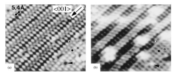
Fig. 20. STM topographic image (a) and simultaneously recorded forward BEEM image (b) on the Si-rich  $CoSi_2/n-Si$  (100) surface ( $V_t = 1.5 \text{ V}$ ,  $I_t = 3 \text{ nA}$ , film thickness d = 38 Å). The center part displays a  $3\sqrt{2} \times \sqrt{2} R45^\circ$  reconstruction, whereas the lower right is  $\sqrt{2} \times \sqrt{2} R45^\circ$  reconstructed. The  $\sqrt{2}$  topographic corrugation is 0.15 Å. The BEEM contrast ranges from 25 pA (black) to 55 pA (white) [98].
