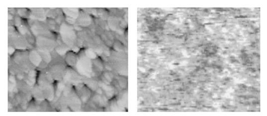
Fig. 34. STM topography/BEEM image pair for a Au/GaN sample. The topography of the Au surface was obtained at  $V_t = 0.5$  V,  $I_t = 1$  nA, and the BEEM image was recorded at  $V_t = 1.8$  V,  $I_t = 2$  nA. Topographic height range is 9 nm, and  $I_c$  ranges from about 0.2 to 2 pA; imaged area is 190 × 160 nm [137].
