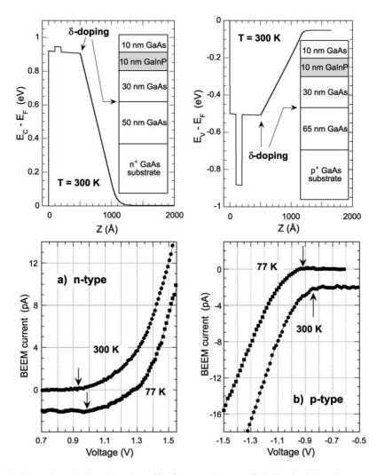
Fig. 41. Upper panel shows the calculated band profiles for n- and p-type  $GaInP_2$  single barrier structures (the MOCVD layer structures are given in the inserts). Lower panel shows representative BEEM spectra (points) for (a) n- and (b) p-type samples containing  $GaInP_2$  layers grown at 610°C. Lines are fits to the BK model to determine the thresholds, indicated by arrows. Curves offset by 2 pA for clarity [169].
