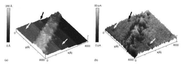
Fig. 46. (a) 3D topographic image of a single quantum wire ( $V_t = 1.8 \text{ V}$ ,  $I_t = 5 \text{ nA}$ ). (b) Simultaneously measured BEEM current image. The arrows indicate accumulated Au clusters in the etched region [37].
