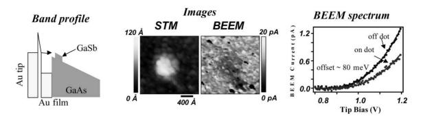
Fig. 49. (from left to right) Schematic of band profile, STM and BEEM images, and characteristic BEEM spectra for GaSb/GaAs self-assembled single quantum dots [39].
