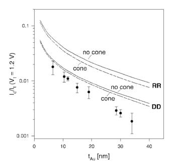
Fig. 19. The value of the BEEM characteristics  $I_c/I_t$  at the tunneling voltage of 1.2 V versus the Au film thickness  $t_{Au}$  for Au/Si(001). Curves are calculated for reflecting (RR) or diffuse (DD) interface structure as indicated by assuming an isotropical Fermi surface ("no cone", *solid line*) and a forbidden cone in the Fermi surface ("cone", *dashed line*). Measured data points are taken from Ref. [55] (from Ref. [53]).
