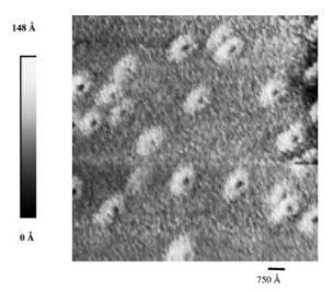
Fig. 47. STM image of surface features in a region where several InAs quantum dots are present and capped with a 50 Å GaAs layer and 85 Å Au layer. The dips near the center of each feature represent the positions of the dots beneath the surface [38].
