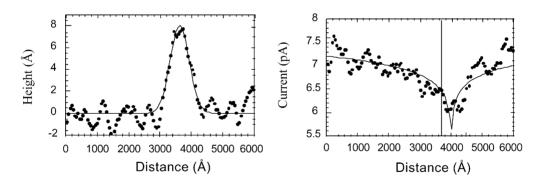
Fig. 28. STM (left) and BEEM (right) linescanes taken over dislocation images. The STM linescanes show a Gaussian peak while the BEEM linescanes show a drop in the BEEM current shifted from the peak in the STM image [112].
