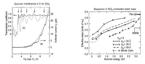
Fig. 56. (a) BEEM spectrum  $I_c V_t$  for 1.8 nm W/3.0 nm SiO<sub>2</sub>/p-Si(100) MOS structure (dotted curve), with  $I_c^0$  shown by a dashed line. (b) Experimental transmission coefficient,  $t(E) = I_c/I_c^0$  (dotted curve), compared to t(E) calculated with a dispersive mass (solid curve). Vertical arrows mark QI maxima for t(E) calculated with a fixed mass  $m_{ox} = 0.42 m_0$ . The threshold is at 3.77 V [205].
