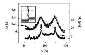
Fig. 21. STM topography (top) and BEEM (bottom) cross sections perpendicular to two parallel dislocation lines, together with a schematic drawing (inset) ( $V_t = 1.5$  V,  $I_t = 2$  nA, film thickness d = 30 Å) [77].
