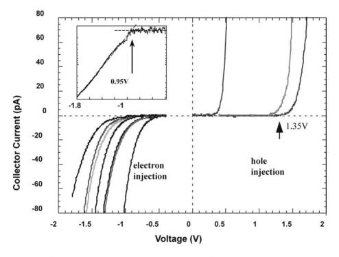
Fig. 33. BEEM spectra for electron and hole injection. Log-plots like the one shown in the inset were used to approximately determine the threshold voltage necessary for current injection into the high-current areas [18].
