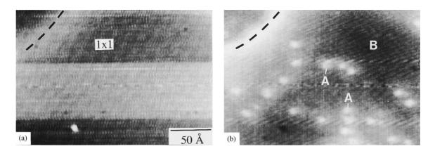
Fig. 45. STM topography (a) and BEEM image (b) of a  $32 \text{ \AA CoSi}_2/\text{n-Si}(111)$  film. The corrugation in the STM topography image is not due to the unreconstructed  $(1 \times 1)$  atomic surface structure but due to small mechanical vibrations. The BEEM current is enhanced at individual interfacial dislocations (dashed line) and subsurface point defects (A) due to hot carrier scattering. ( $V_t = 1.8 \text{ V}$ ,  $I_t = 10 \text{ nA}$ ) [81].
