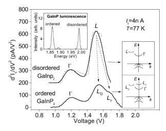
Fig. 37. SD-BEEM spectra for two GaAs/GaInP<sub>2</sub> (ordered and disordered) samples with 50 Å GaAs cap layers, taken at T = 77 K. For clarity, the spectra are shifted along the vertical axis. The MSIS model calculations are also presented (dashed line). The top inset shows the photoluminescence spectra for both ordered and disordered GaInP<sub>2</sub> samples, whereas two bottom insets show the schematic of the GaInP<sub>2</sub> band structure [16].
