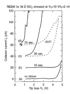
Fig. 55. A successful breakdown sequence for a 3.8 nm oxide stressed with 6 eV (kinetic energy) electrons. The shift to higher  $V_s$  between curve (a) and (b) is due to negative charge at the SiO<sub>2</sub>–Si interface. Total injected charge to breakdown (defined by reaching  $V_s \sim 1$  V, as in curve (c) is  $\sim 6 \times 10^{13}$  C/cm<sup>2</sup> [201].
