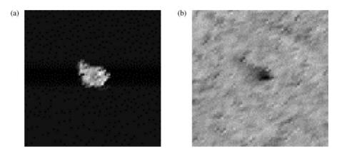
Fig. 32. Collector current image (a) and simultaneously taken STM image (b) of the 70 Å Au cap layer of a 2500 Å × 2500 Å area ( $I_t = 1$  nA,  $V_t = -1.8$  V). The small high-current area (~ 500 pA, bright spot) surrounded by areas with zero collector current (< 0.2 pA) shown in (a) is typical for the investigated GaN-films. The Au layer (right) exhibits a pit (dark) at the location of the high-current area (bright spot (a)) [18].
