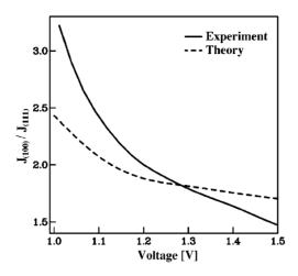
Fig. 18. Ratio of current injected in Si(100) and Si(111) after propagation through thin Au films of approximately equal thickness (100Å Au/Si(100) and 75 Å Au/Si(111), chosen to compare with available experimental data). Elastic electron propagation is used in the theory (dashed line); experimental data taken from Refs. [86,96] (solid line) [95].
