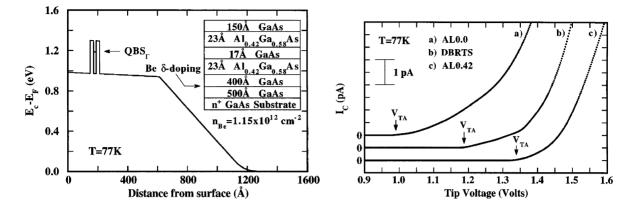
Fig. 42. Left panel shows the layer structure and calculated band profile of the DBRTS structure whose design included the  $\delta$ -doped Be sheet to flatten the band profile at room temperature. Right panel shows the BEEM spectra at 77 K for (a) the reference GaAs sample, (b) DBRTS, and (c) GaAs/Al<sub>0.42</sub>Ga<sub>0.58</sub>As single barrier sample [33].
