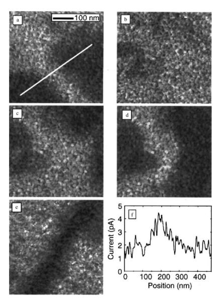
Fig. 51. (a)–(e) BEEM images (500 × 500 nm<sup>2</sup>) taken at a fixed position in a varying magnetic field applied parallel to the film plane, (a) before the applied field, and in applied fields of (b) -40 Oe, (c) 10 Oe, (d) 20 Oe, and (e) 40 Oe. The linear gray-scale range for each is from 1.0 pA (black) to 5.0 pA (white).  $V_t = 1.5$  V and  $I_t = 2$  nA. (f) is a cross-sectional view of the position indicated in (a) [184].
