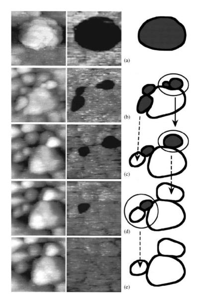
Fig. 31. Series of STM (left) and BEEM (middle) images during an erasing process of the Au/Si(1 1 1) interface. (a) Images taken before the process and (b)–(e) images taken after every scanning with a positive voltage of 1.34 V. The size of the images is 47 nm  $\times$  47 nm. Schematics shown on the right demonstrate a variation of Au grain structures with the BEEM current contrast together [121].
