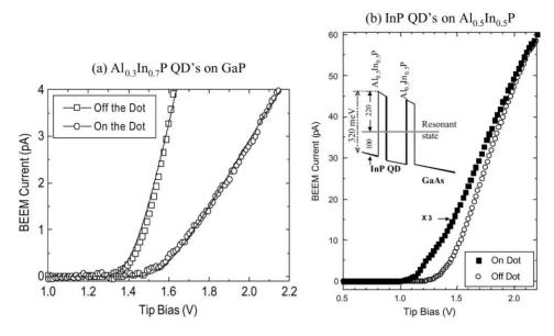
Fig. 50. BEEM current spectra taken on and off the QD for the case of (a)  $Al_{0.3}In_{0.7}P$  QDs on GaP and (b) InP QDs on  $Al_{0.5}In_{0.5}P$  grown on a GaAs matrix. A band diagram is shown in the inset [40,182].
