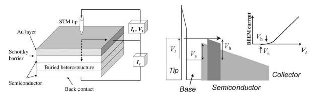
Fig. 1. A schematic of BEEM experimental setup.
