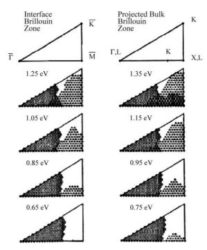
Fig. 7. Phase space for electron transmission through a  $CoSi_2/Si(111)$  interface. The panels show the irreducible wedge of the interface Brillouin zone of both  $CoSi_2$  and the Si. At each parallel wave vector used in the calculation there is an open circle if there is at least one state at that energy in the  $CoSi_2$  and a plus if there is at least one state in the Si. If there is a state in both, the open circles fill in and become closed circles [76].
