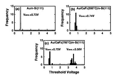
Fig. 54. Distributions of measured threshold voltages of (a) 25 ML Au/Si(111), (b) 50 ML Au/2 ML  $CaF_2$  (550°C)/Si(111), and (c) 50 ML Au/2ML  $CaF_2$  (700°C)/n-Si(111) [199].
