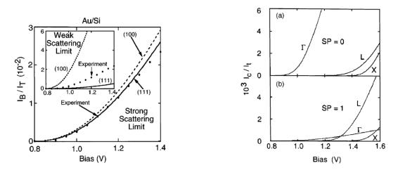
Fig. 10. Comparison of the calculation in the strong scattering limit for Au/Si(100) (dashed line) and Au/Si(111) (solid line) with the experimental results for Au/Si of Refs. [86,87]. These measurements were made on Au/Si(111) but measurements for Au/Si(100) are very similar to those for Au/Si(111) (see Refs. [70,102]). The inset (referenced earlier in our paper as Fig. 6(a)) compares the calculation in the weak scattering limit to the same experimental results [85].
