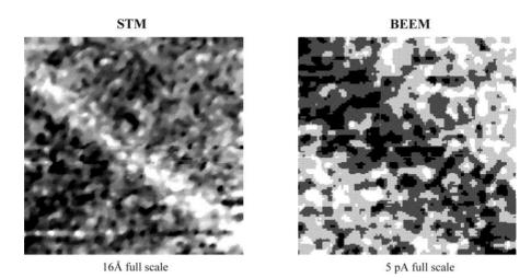
Fig. 27. 1  $\mu$ m × 1  $\mu$ m STM (left) and BEEM (right) images of In<sub>x</sub>Ga<sub>1-x</sub>As/GaAs heterostructure (x = 0.2, d = 600 Å). The STM image shows the growth perturbation caused by the dislocation core. The BEEM image shows the decrease in current at the presence of the cross-hatch [112].
