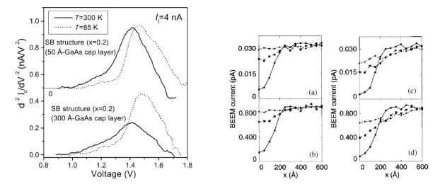
Fig. 25. SD-BEEM spectra for GaAs/Al<sub>0.2</sub>Ga<sub>0.8</sub>As/ GaAs single barrier (SB) samples with 50 and 300 Å GaAs cap layers, taken at T = 300 K (solid curves) and T = 85 K (dotted curves). For clarity, the spectra are shifted along the vertical axis [5].
