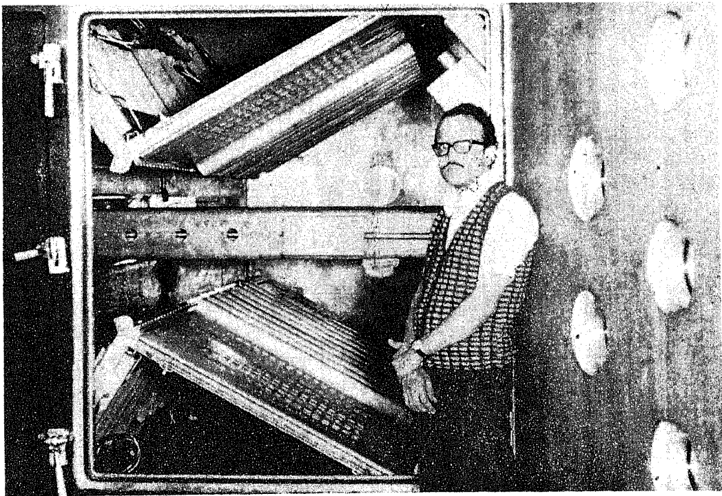
Figure 7. Radiofrequency movable panels and the dee stem inside the resonator tank.
