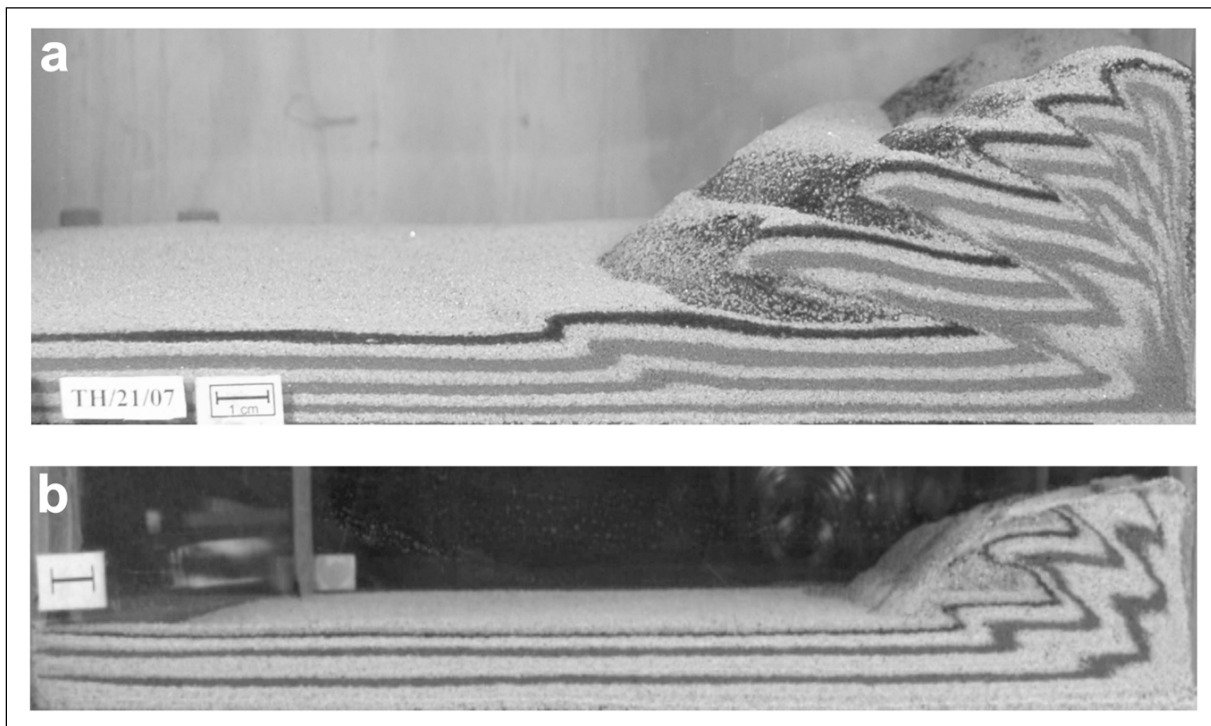
Fig.2. Thrust sequences in sand models with high basal friction ( \mu_b = 0.46 ). (a) Model with no erosion. (b) Model with syn-thrusting erosion. Note that frontal thrusts in (a) show a strong variation in their spacing, whereas the spacing remains more or less uniform in (b). Models were deformed by horizontal contraction (right to left). Scale bar: 1 cm.
