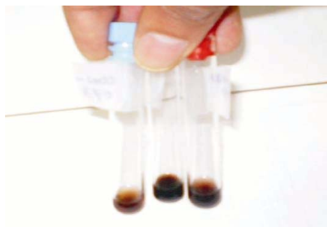
Figure 1. A photograph of the steroid capped gold nanoparticle dispersions (1, 2 and 3 capped NPs from right to left).
