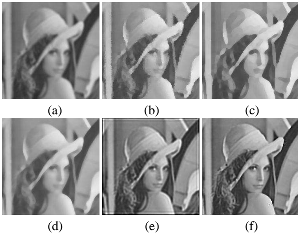
Figure 3: Result of inverse diffusion of (a) the blurred Lena image using (b) Osher-Rudin shock filter, (c) Alvarez-Mazorra shock filter, (d) Gilboa et al. complex shock filter, (e) Lucy-Richardson deconvolution and (f) gradient based cluster separation shock filter.
