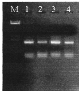
FIG. 4. Amplification of SRY from human male DNA. Lane M: \lambda DNA digested with the enzyme Hind III (molecular size DNA marker), Lane 1 and 3: PCR products obtained from PTC-150 (MJ Research), Lanes 2 and 4: PCR products obtained from the induction heating-based thermocycler (present study). The size of the PCR products is 840 bp.
