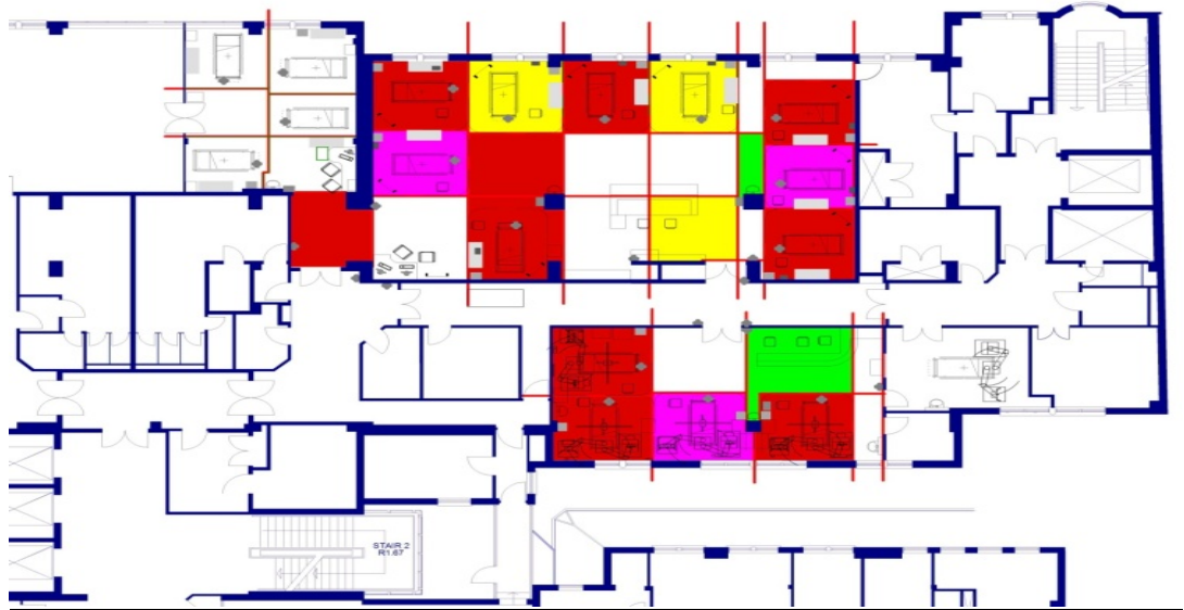
Figure 3-1 Mean number of CFUs detected at level 0 in bed spaces and SITU and MITU ward areas over a 3 month period on sampling sites under 0.6m (green areas <50 CFUs, yellow areas 50 -100 CFUs. pink areas 101 and 200 CFUs, red areas over 200 CFUs).
