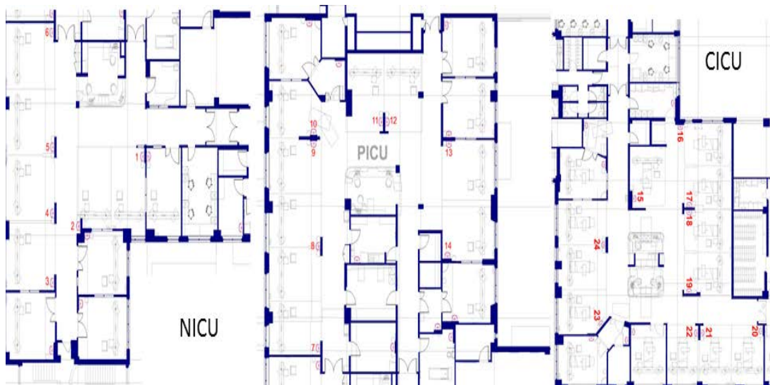
Figure 2-3 Floor plans for CICU, NICU and PICU at GOSH with sink locations labelled and numbered in red.
