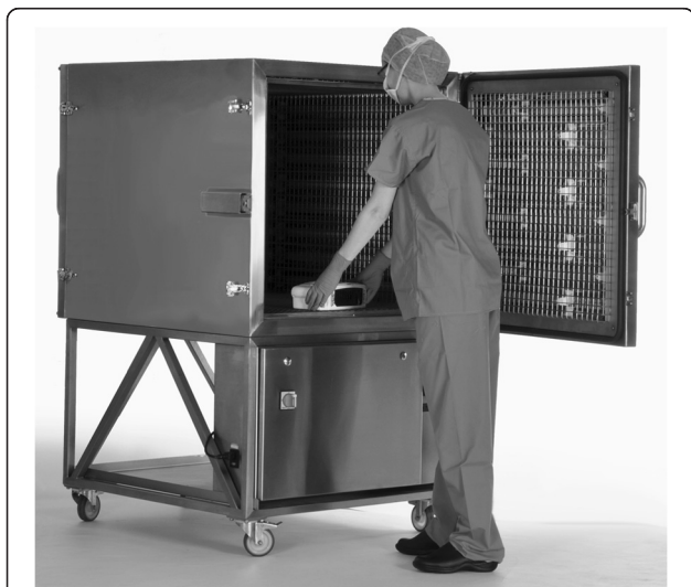
Figure 4 Placing an item to be disinfected inside the Nanoclave Cabinet.
