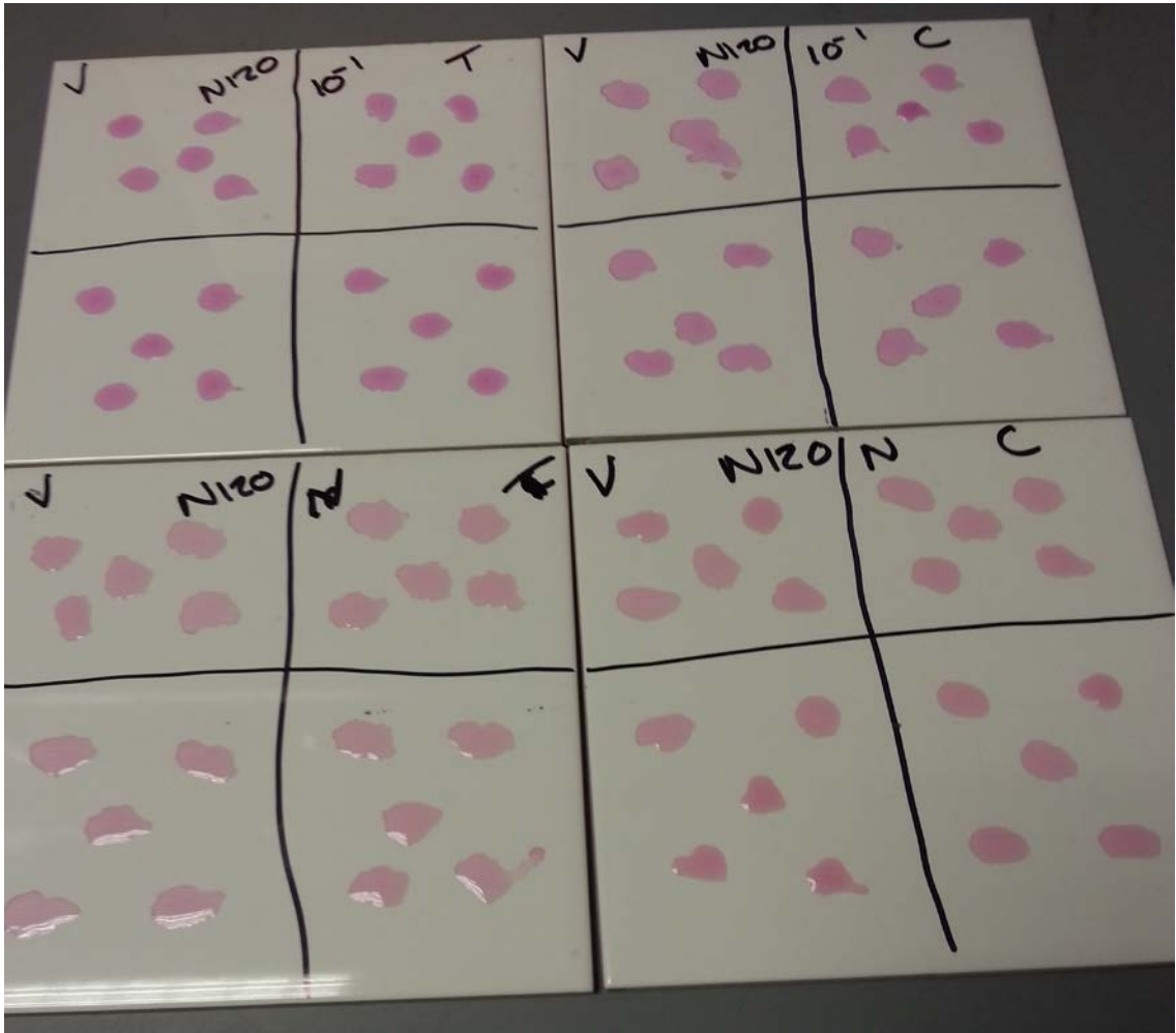
Figure 2-2 Ceramic tiles inoculated with 250µl of suspension per replicate in 50µl droplets, with four replicates per tile.
