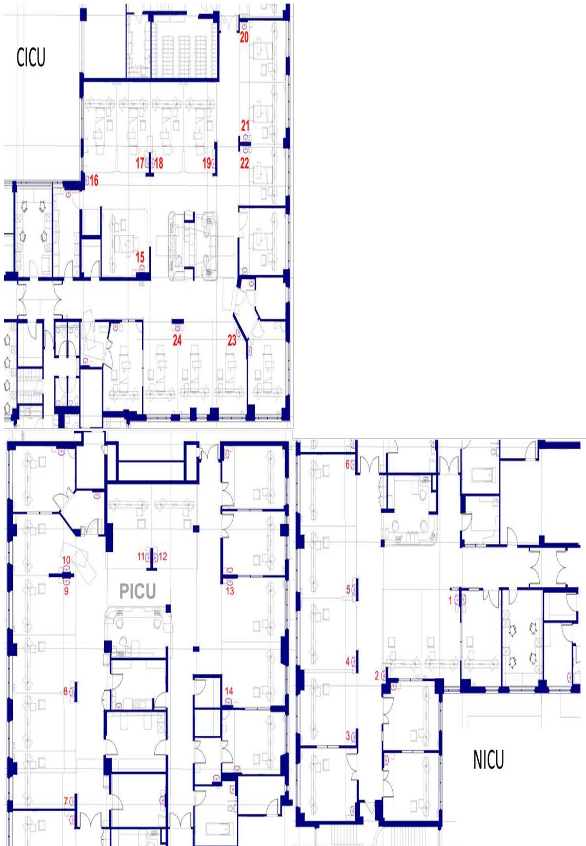
Figure 5-13 GOSH floor plans for areas studied (PICU, CICU and NICU) showing numbered sink locations.
