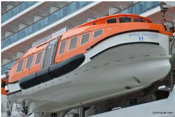
Figure 2.1 Partially enclosed lifeboat
