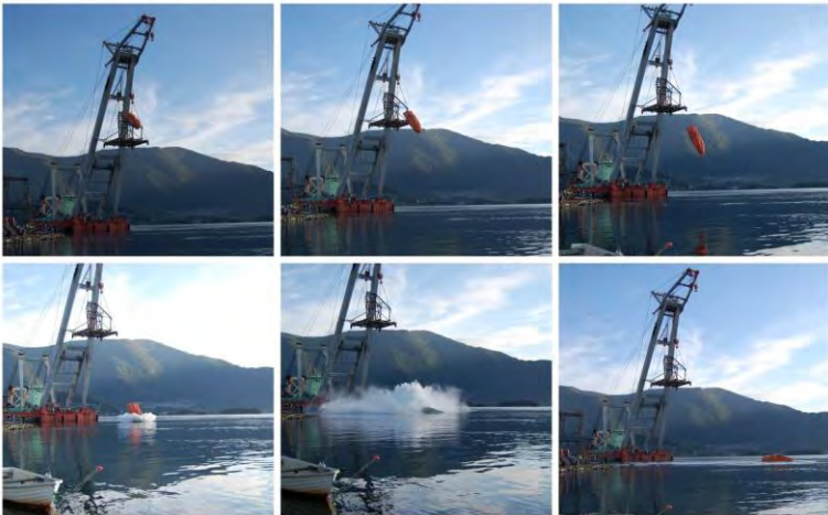
Figure 2.5 Full scale free fall lifeboat trial
