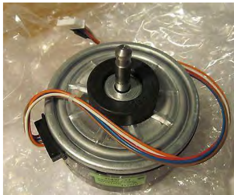
Gambar 3.3 Motor BLDC Daikin D43F [3]
