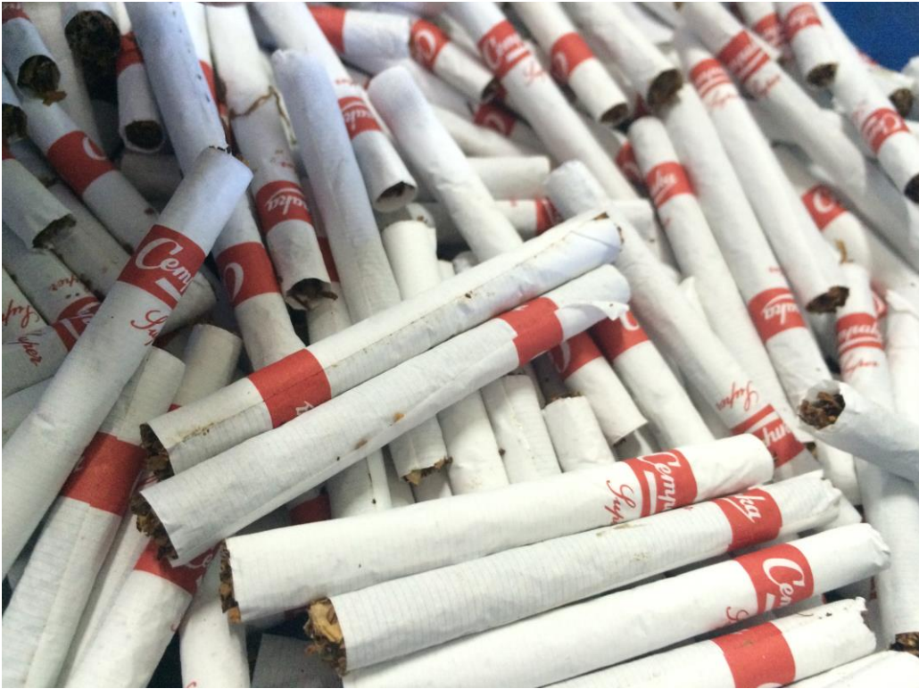
APPENDIX D: Uneven Size Defect
