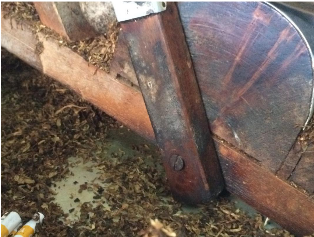
APPENDIX G: Loose Bolt in the Rolling Tool
