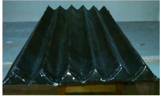
Figure 5. Photograph of the triangular waveform absorber plate
