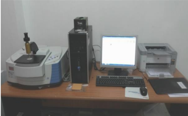
Gambar 3.8 Alat uji FTIR
