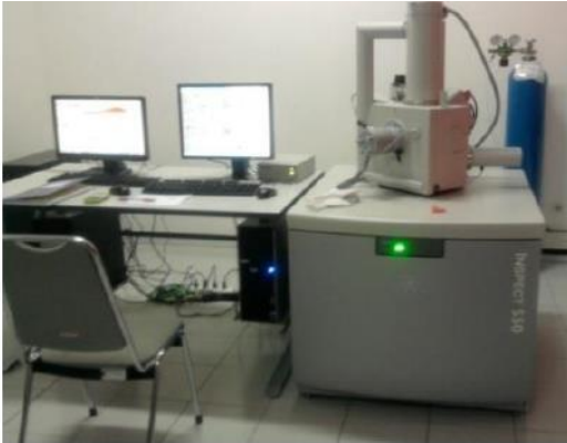
Gambar 3.4 Scanning Electron Microscopy (SEM) Jeol JSM-7001F Inspect S50 23
