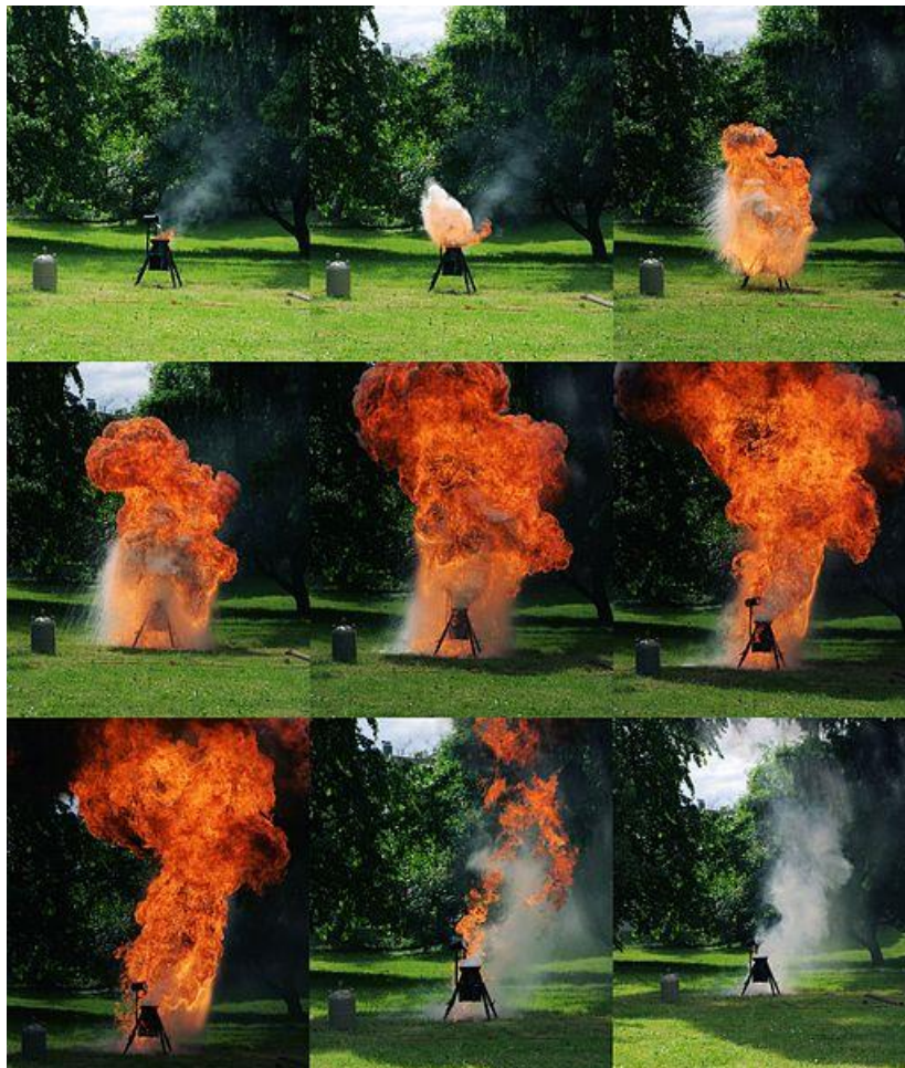
Figure 2.1. Simulation of boil over is performed in small scale. one kilogram of cooking oil was poured with 1 liter of water. source picture: Wikipedia, 2017
