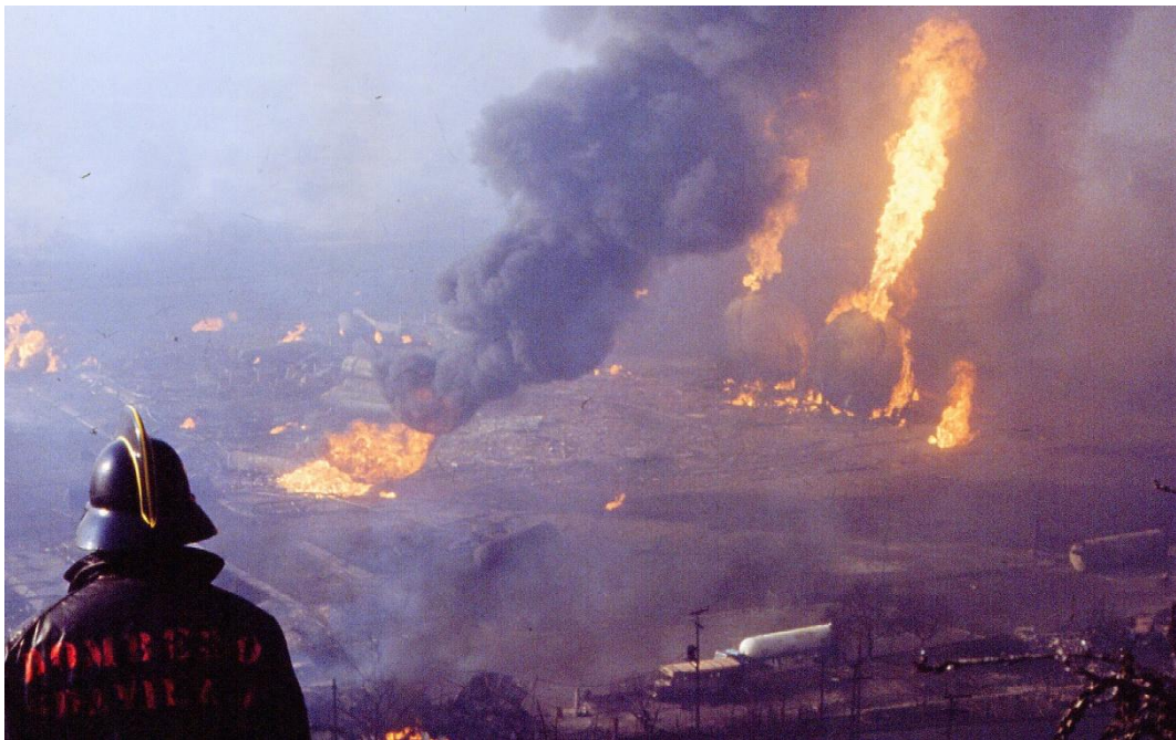
Figure 2.2. Example of BLEVE during San Juanico disaster, 1984. source picture: alchetron.com
