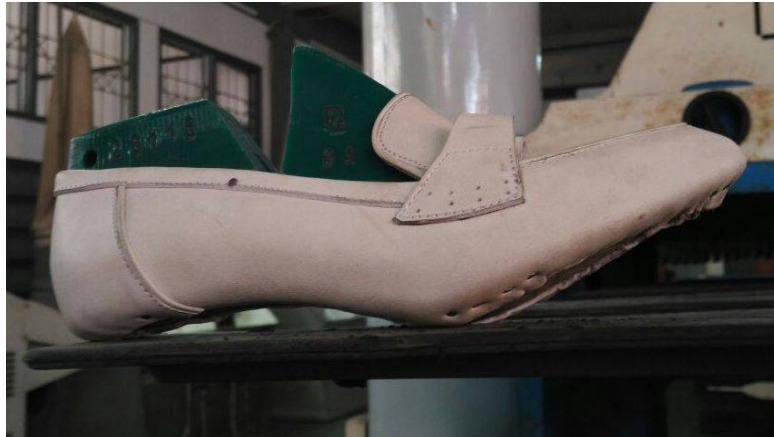
Gambar 4.9 Hasil Proses Lasting
