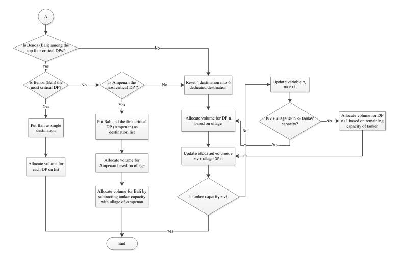
Figure 5. 5 Conceptual Model for Selecting Discharge Port (cont'd)
