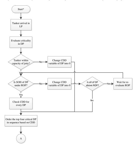
Figure 5. 4 Conceptual Model for Selecting Discharge Port
