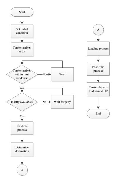
Figure 5. 3 Conceptual Model for Loading Mechanism
