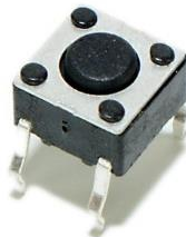
Gambar 2.20 Push Button Switch [18].
