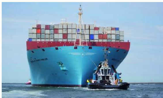
Gambar 2.4. Towing Tugboat (Sumber: http://products.damen.com/-/media/Products/Images/Clusters-groups/Tugs/harbour_tug.jpg?h=767&la=en&w=1300 )
