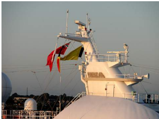
Gambar 2.9. Box Girder and Frame Work Mast (Sumber: http://www.beyondships.com/images/xu_mast.jpg )
