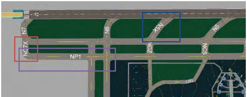
Gambar 5.2 Perpanjangan Taxiway NP1 Sisi Barat, Penambahan Rapid Exit Taxiway N5X dan Taxiway N7X
