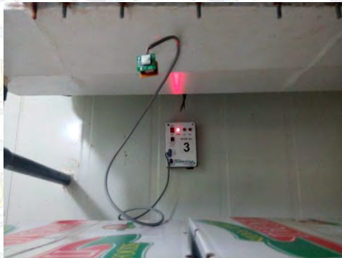
Figure 4.12. Sensor Node Located in the Top Side of Cold Storage
