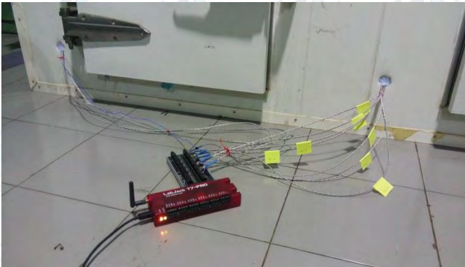
Figure 4.25. Labjack T7 Pro Installation during Experiment
