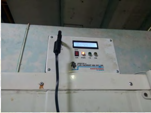
Figure 4.13.Coordinator of WSN System
