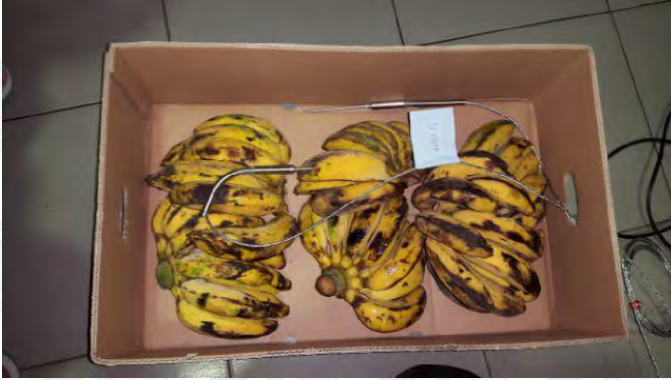
Figure 4.20. Thermocouple Placement in the Cargo
