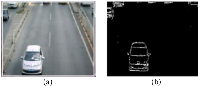
Gambar 4.7 Citra hasil Background Subtraction dengan metode Improved Three Frame Difference . (a) citra asli, (b) citra foreground .
