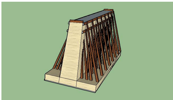
Gambar 4. 91 Bekisting landhope pelimpah
