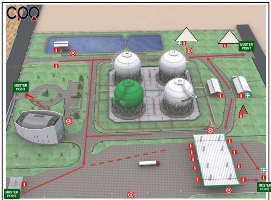
Figure 4.4 Terminal Fire Fighting Arrangement
