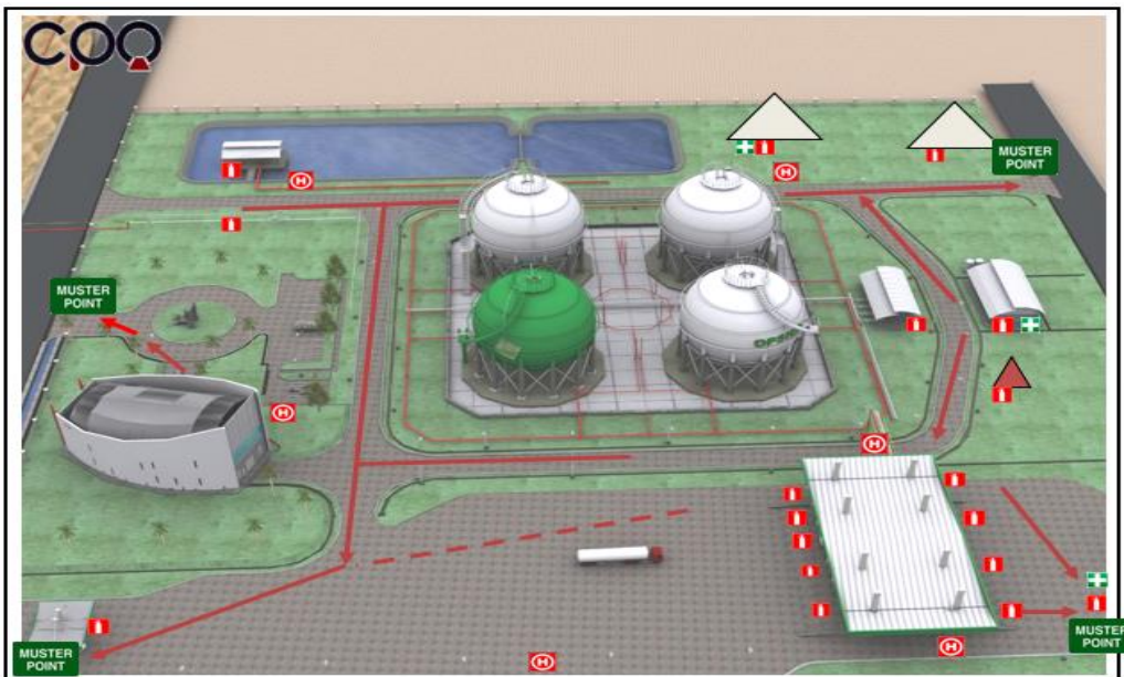
Figure 10.1. Location of the Fire Extinguisher at Terminal LPG Semarang
